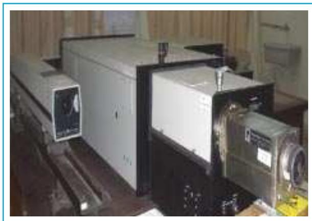
Laser Raman Spectrometer has been installed at the Institute in November 2005. It is a double monochromator spectrometer. Argon ion laser is used as source. It will operate at two wavelengths 514.5 nm in green region and 488.0 nm in blue region. This system will be used to investigate the molecules present in a particular sample and chemical composition of aerosols collected from different atmospheric conditions.
