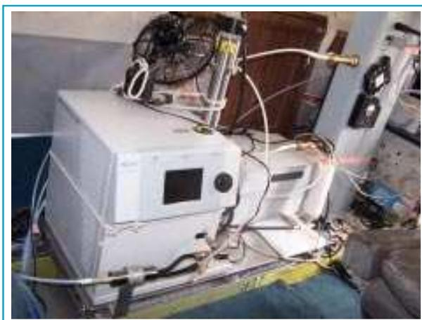
*Installation of Scanning Mobility Particle Sizer (SMPS) onboard the aircraft during ICARB*
