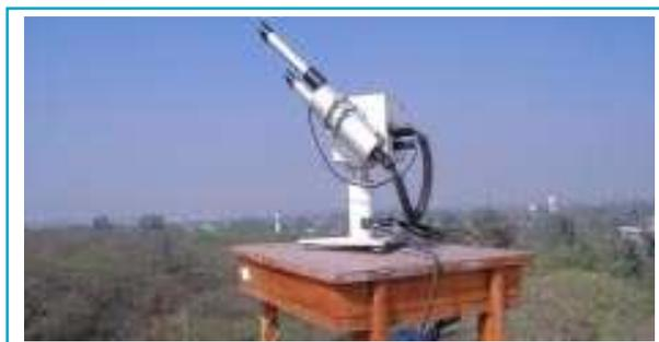
An automatic sun tracking sun/sky radiometer (Prede Model POM-01L) has been installed at the IITM New Delhi Branch on 17th February 2006 to monitor aerosol optical properties at the urban location under the ICARB Campaign.
