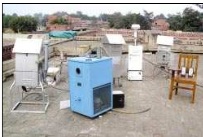
Aerosol samplers, fog water collector and MICROTOPS II operated by IITM at Agra during the Nation-wide Land Campaign II
