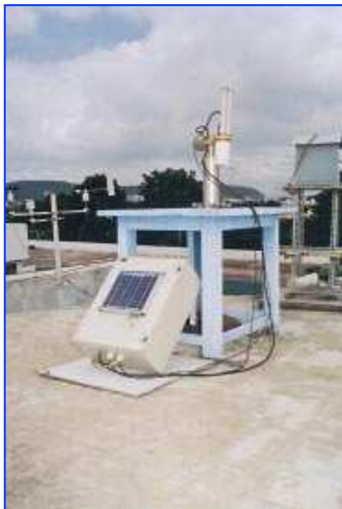
CIMEL polarized Sun and Sky Radiometer installed at the IITM, Pune for atmospheric aerosol characterization experiments. Solar panel for auto power to the instrument and control unit is seen in a box below the Radiometer
