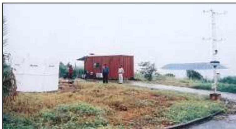
From L to R: Mini-Sodar of Indira Gandhi Centre for Atomic Research Laboratory and Tower with Meteorological Sensors of the IITM
