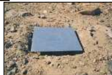
Plate antenna for Air-Earth current
