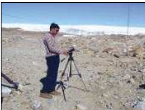
Multichannel sunphotometric and ozonometric measurements of aerosols and gases over Maitri
