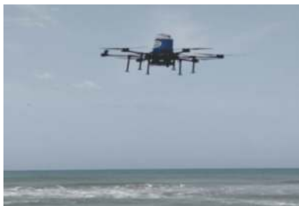
Fig. 30 : (a) Testing of IITM mGHG gas sensor system on a Hexacopter. (b) Drone experimentation at ART-Bhopal
