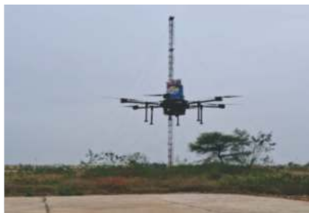
Fig. 30 : (a) Testing of IITM mGHG gas sensor system on a Hexacopter. (b) Drone experimentation at ART-Bhopal
