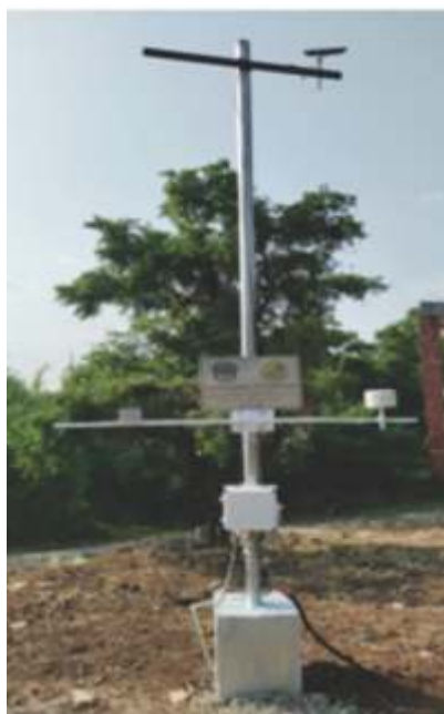
a) Installation of an Eddy Covariance system ( \text{CO}_2\text{-H}_2\text{O} sensor, Sonic Anemometer) at the ARIES-Nainital campus. Furthermore, b) installation of an Eddy Covariance system ( \text{CO}_2\text{-H}_2\text{O} sensor, \text{CH}_4 Sensor, Sonic Anemometer) along with weather sensors at the Pichavram Mangrove site.
