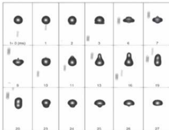
Fig. 20: Sequence of high-speed camera images showing coalescence after the collision of drop pair ( dL=3.27\text{mm} ; dS=0.789 \text{ mm} ) in the presence of EH=300 \text{ kVm}^{-1} . The time shown indicates the evolution of breakup in ms. The smaller drops seen in the top/bottom/left side of the picture are not part of the coalescence.
