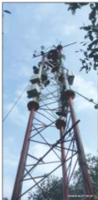
a) Installation of an Eddy Covariance system ( \text{CO}_2\text{-H}_2\text{O} sensor, Sonic Anemometer) at the ARIES-Nainital campus. Furthermore, b) installation of an Eddy Covariance system ( \text{CO}_2\text{-H}_2\text{O} sensor, \text{CH}_4 Sensor, Sonic Anemometer) along with weather sensors at the Pichavram Mangrove site.
